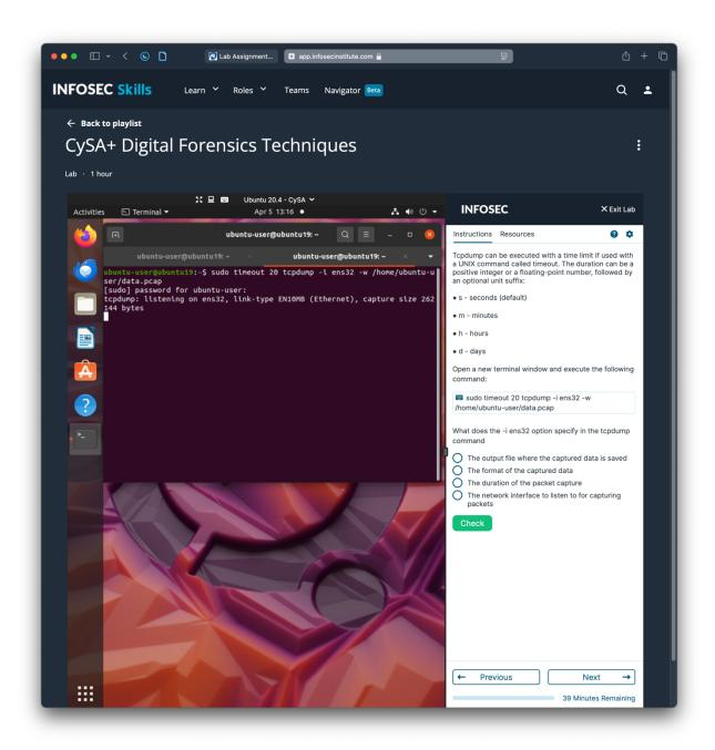
Figure 4. Running tcpdump with a 20-second time limit.
