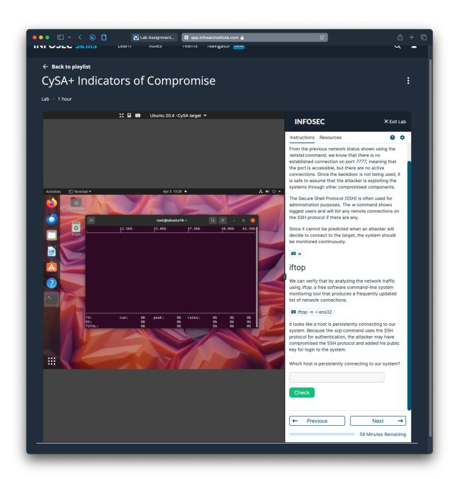
Figure 8. Monitoring network traffic with iftop.
