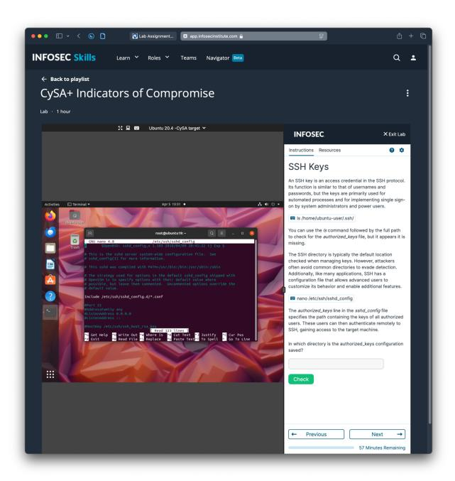
Figure 9. Examining the SSH server configuration file.
