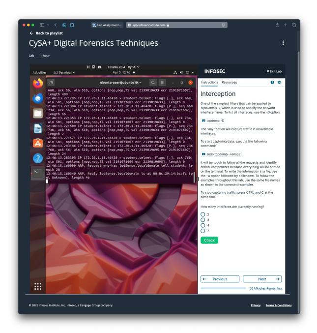
Figure 3. Capturing traffic with tcpdump.
